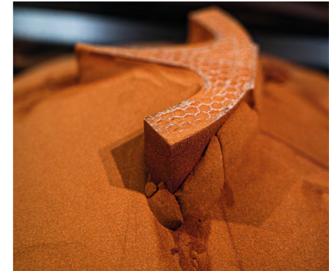
Component for accelerators made from copper powder using 3D printing for the first time.
